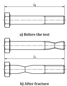
Figure 6 — Determination of elongation after fracture, A
